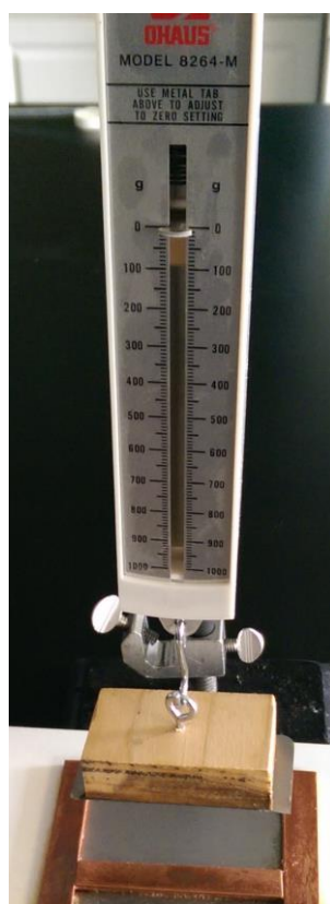
Figure 3: Test apparatus used for the pull-off experiment.
