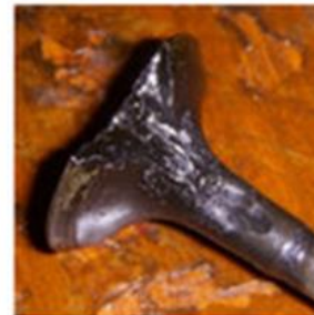
Exhaust valve melt
