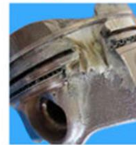
Piston ring land crack
