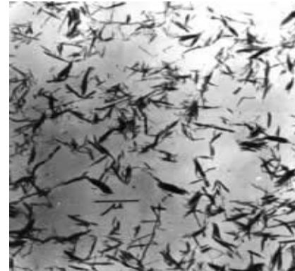
Electron microscopy micrograph of soap particles in a sample of lubricating grease
