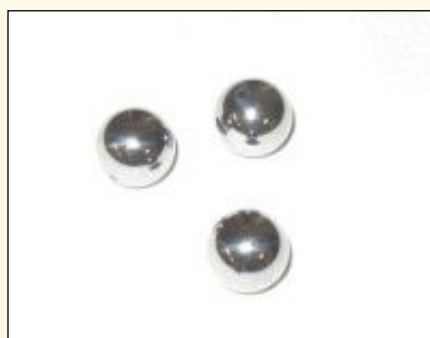
Figure 7 | Good EP performance means that a grease will prevent the 52100 steel balls from welding. (Courtesy of TriboScience & Engineering, Inc.)
