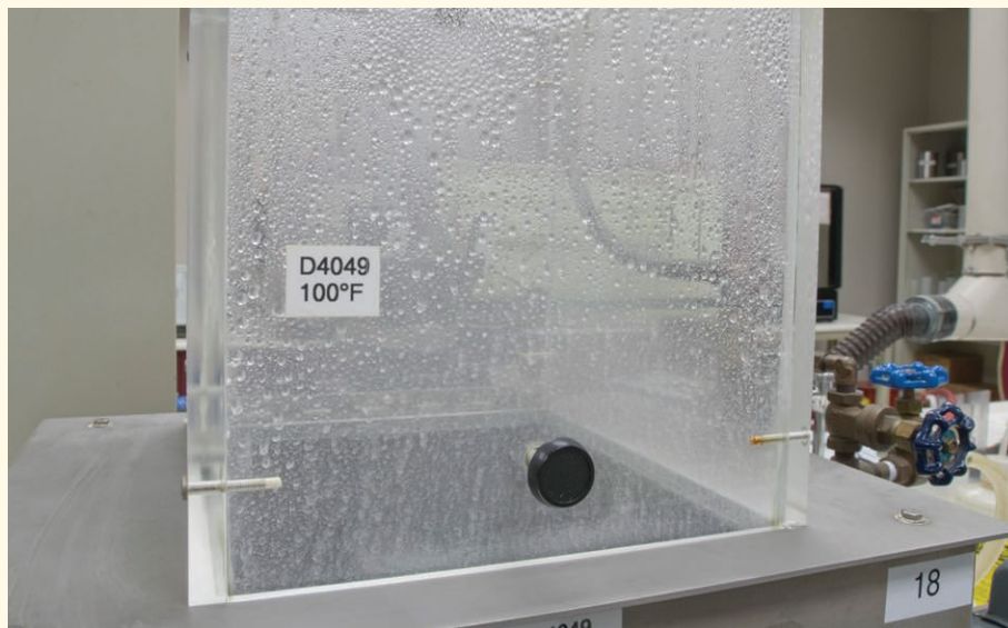
Figure 4 | The ASTM D4049 procedure uses an enclosed booth to direct a spray nozzle on a panel coated with grease to determine the percent spray-off as a measure of water resistance. (Courtesy of The Lubrizol Corp.)
