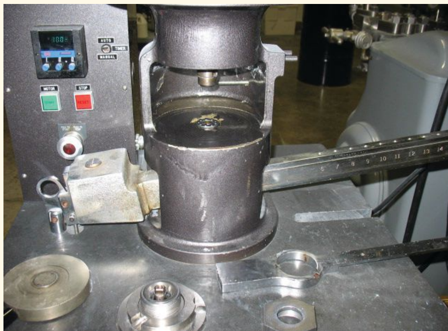
Figure 6 | The tribometer shown is used to evaluate the extreme pressure (EP) properties of a grease. (Courtesy of TriboScience & Engineering, Inc.)
