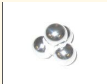
Figure 8 | Frictional heat causes the 52100 steel balls to weld in a poor result. (Courtesy of TriboScience & Engineering, Inc.)
