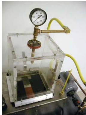
Figure 5 Water spray test setup
